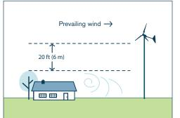
A properly sited Whisper wind generator must be placed 20 ft (6 m) above any surrounding object within a 250 ft (76 m) radius.
